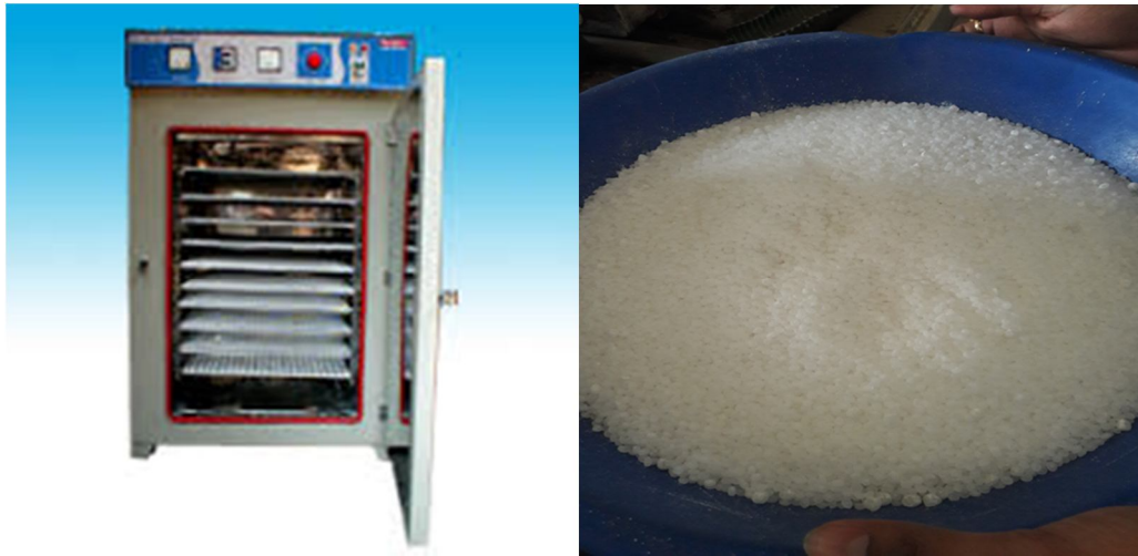
Fig 4.2 Sample after Drying in Tray Drier.
