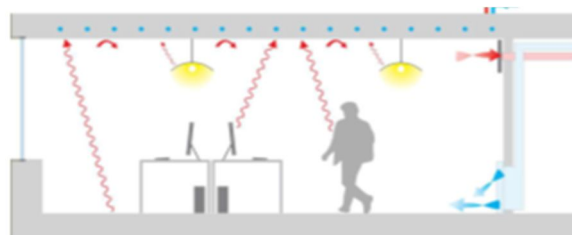
Figure 2.1- radiant cooling from ceiling
