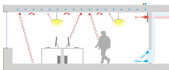
Figure 2.1- radiant cooling from ceiling
