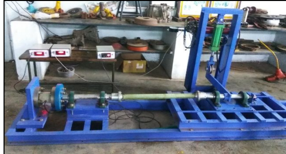
Fig 1-Test rig for torsional strength
