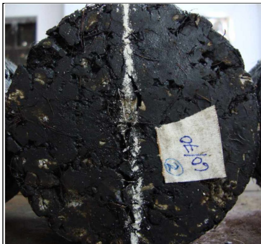
Fig 5.3 Specimen to be tested after adding coir fibre
