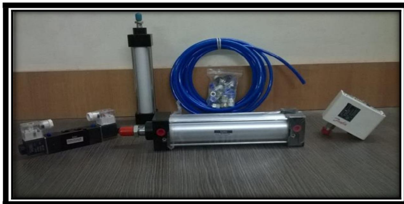
Fig 7. DCV, Cylinders, Pressure switch and pipe etc
