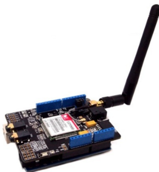
Fig 3. GPRS Shield Interfaced To Arduino Uno
