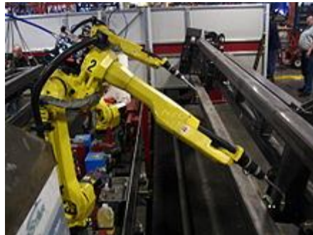
Fig.1 A set o six –axis robot used for welding.
