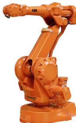
Fig.2 IRB2400 Industrial Robot from ABB
