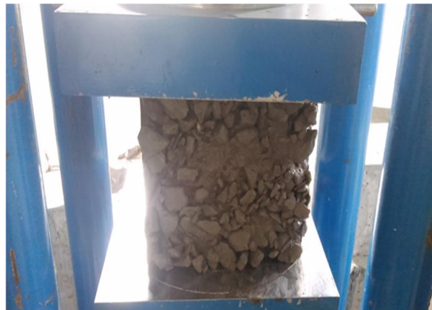
Fig.2: Cube Compressive strength test for prepared cube
