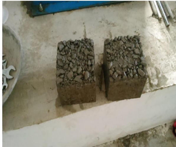
Fig. 1 Prepared cube for compressive strength test
