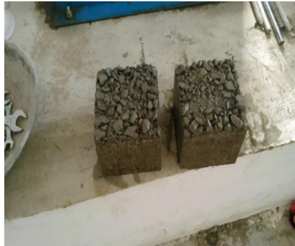
Fig. 1 Prepared cube for compressive strength test
