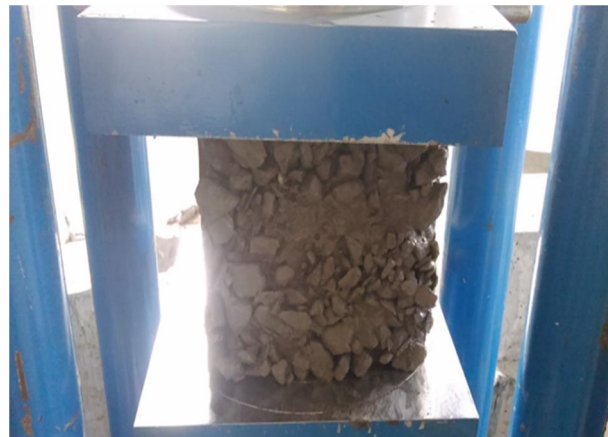
Fig.2: Cube Compressive strength test for prepared cube
