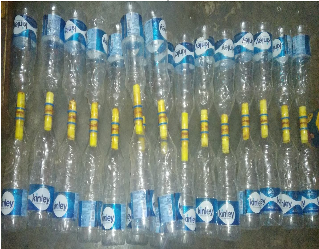
Fig. : 16 Array of Two connected bottles, made with help of plastic pipe to join them
