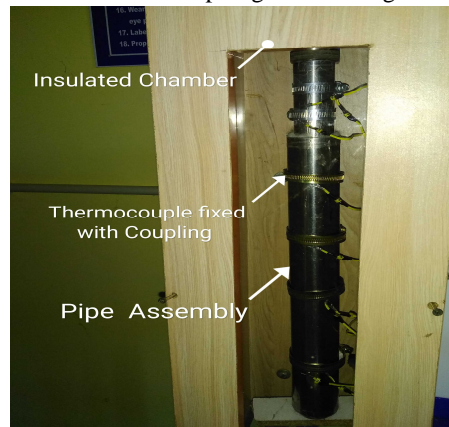
Fig. : Pipe assembly inside experimental chamber. Thermocouples on inner and outer surface
