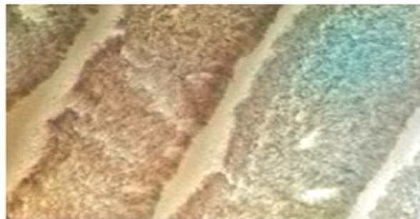
Fig. 1 Photograph of strips of oriented Zinc Oxide and Graphene composites synthesized on a substrate.
