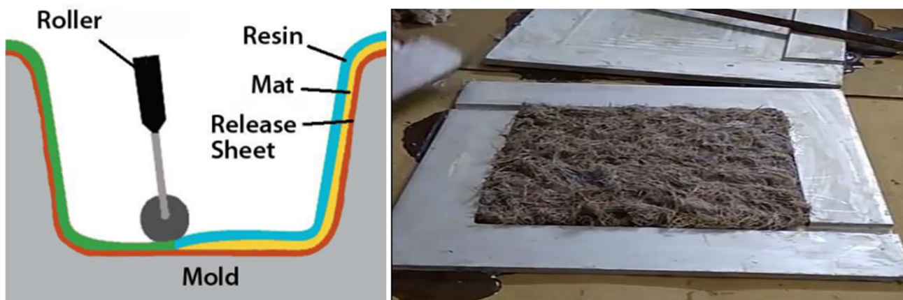
Fig. 3 Fabrication of composite by Hand Layup Technique.
