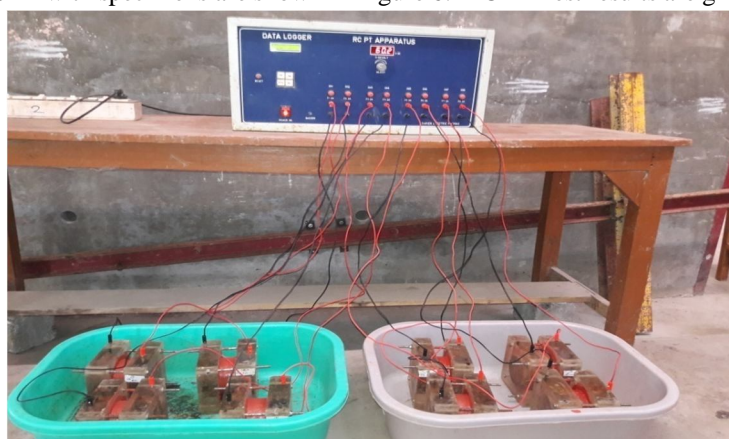
Figure 6. RCPT Test Set up with specimens
