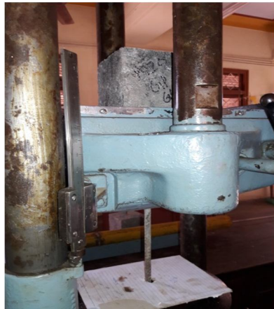
Figure 7. Pull Out Test Set up with specimen
