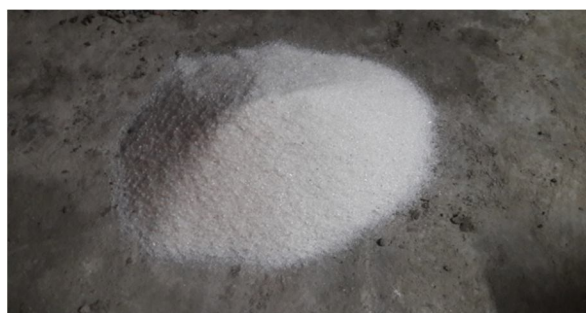
Figure 1. Recycled Waste Glass as Fine Aggregate
