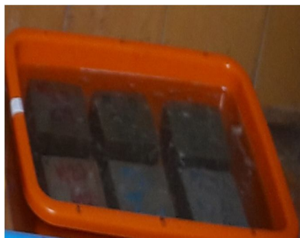
Figure 5. Specimens Immersed in MgSO_4 with Na_2SO_4 Solution
