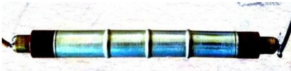
Fig.4: GM Tube Used For Radiation Detector
