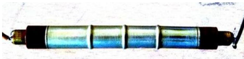
Fig.4: GM Tube Used For Radiation Detector
