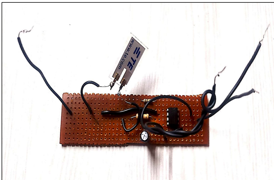
Fig. 6 Circuit of charge amplifier constructed by us
