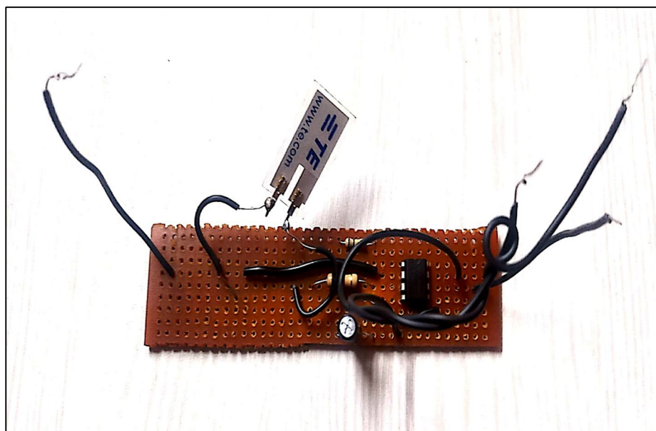
Fig. 6 Circuit of charge amplifier constructed by us
