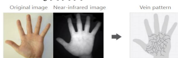
Fig. 2 A Process of extracting Palm vein pattern
