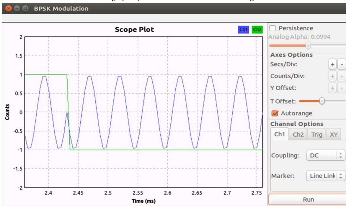
Figure 6: Output waveform of BPSK modulator using GNU radio
