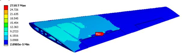
(Magnified view of the stress plots is shown below i.e it represents the maximum stress induced in the frequency 27.817HZ)
