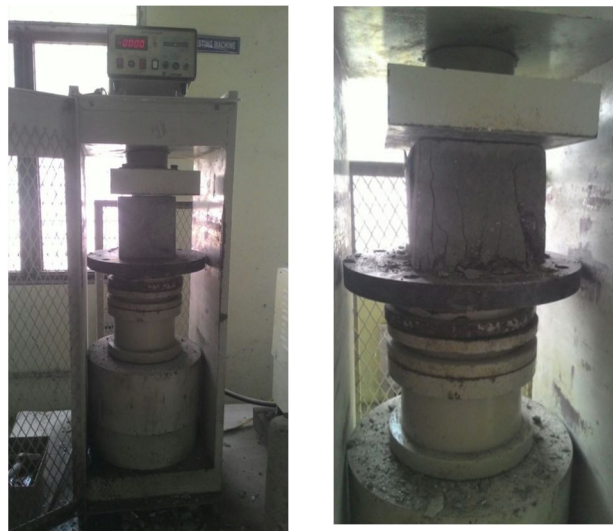
Fig 4.1. Test setup for Compressive strength of Cube
