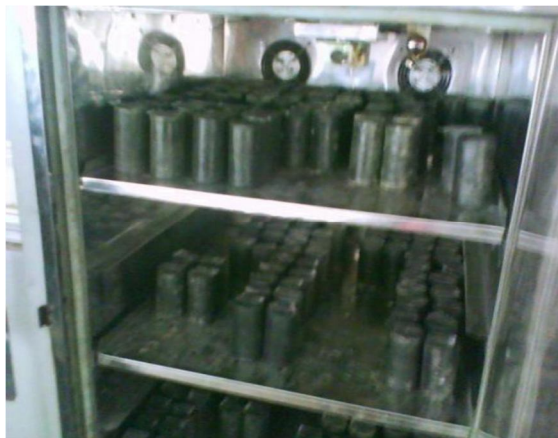
Fig : Lime stabilized fly ash & BFS coated with Wax
