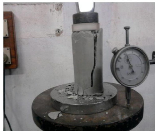
Fig : UCS test on wax coated Lime treated fly ash & BFS
