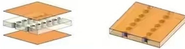
Fig. 4.1 3D representation of SIW structure
