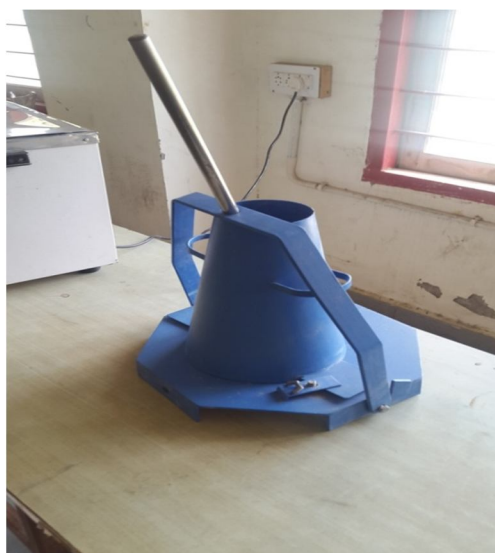
Fig 3.11 Slump Test Procedure
