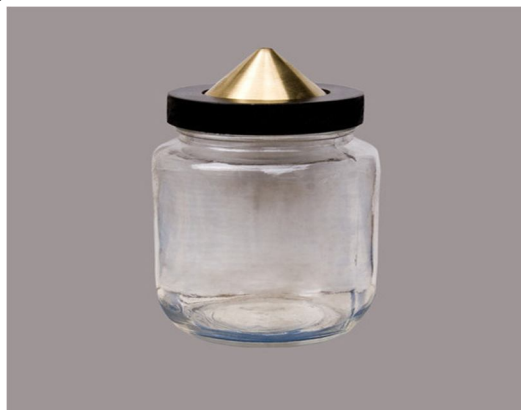
Fig 3.4 Specific gravity of Fly Ash pycnometer
