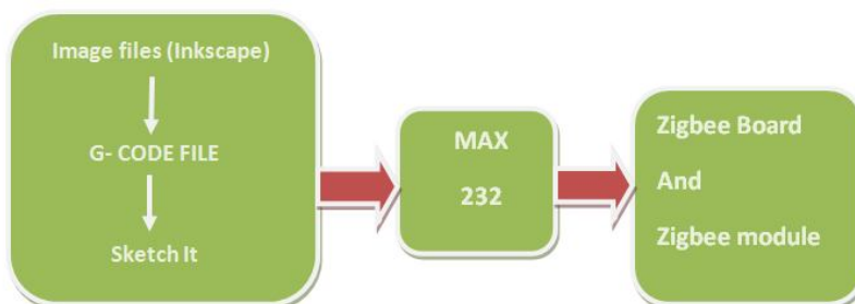
Fig. block diagram of Transmitting side of mini CNC plotter
