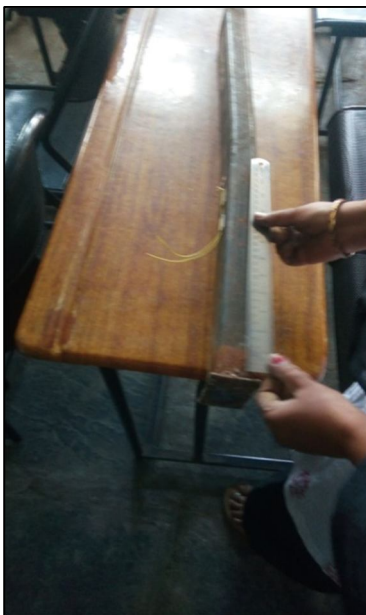
Figure No. 4 Deformed Rectangular CFST Columns after Experiment
