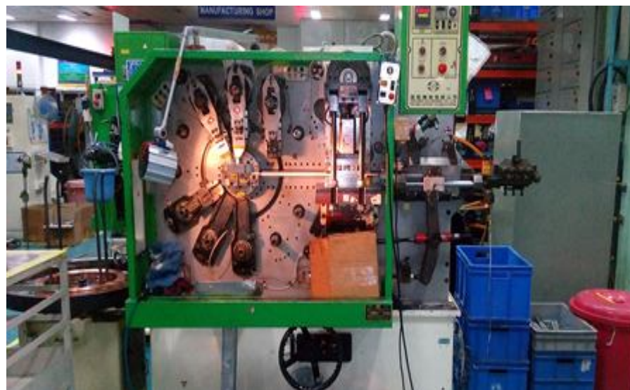
Fig 6: YSM Multislide Machine With Press Tool
