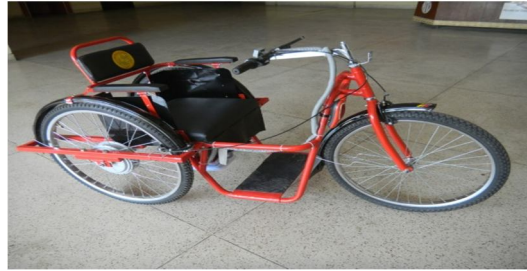
Fig (2); - This is a semi advanced tricycle which runs by electric energy but the disadvantage of this cycle is that this tricycle does not come in reverse direction.
