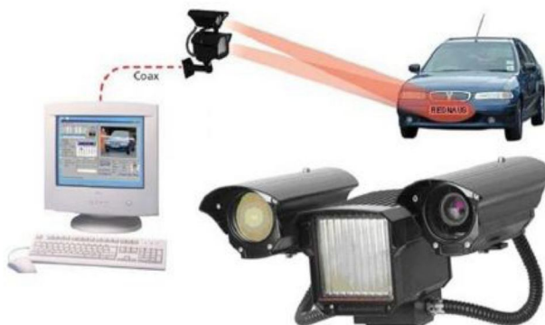
Fig. 1 Hardware components of ANPR
