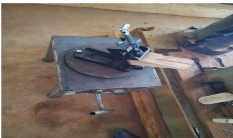
Fig. 3.3 Fabricated model of Rotating and Tilting vice
