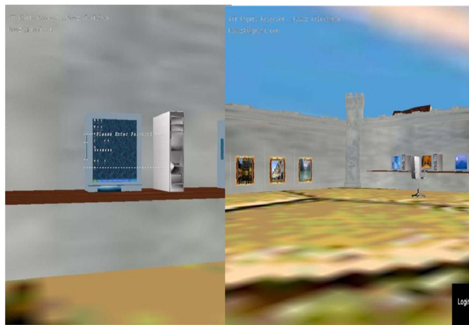
Figure 3 – (a) Snapshot of a proof-of-concept 3-D virtual environment, where the user is typing a textual password on a virtual computer as a part of the user's 3-D password. (b) Snapshot of a proof-of-concept virtual art gallery, which contains 36 pictures and six computers
