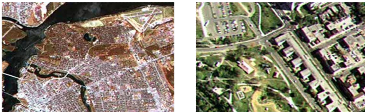
Fig.4 Examples of a coarse resolution and a fine resolution image
