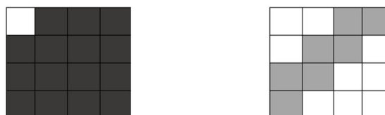
Figure 9 (a) DC and AC Coefficients in 4x4 Block (b) Mid-Band Region of 4x4 block
