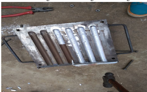
Fig: 5 Casted Specimens
