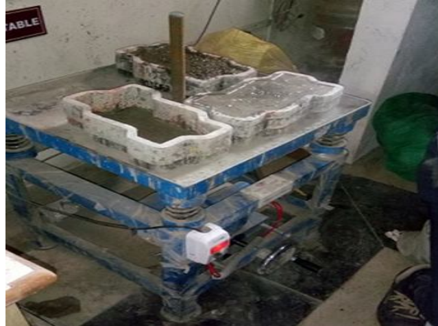
Fig.3 Vibrating of concrete
