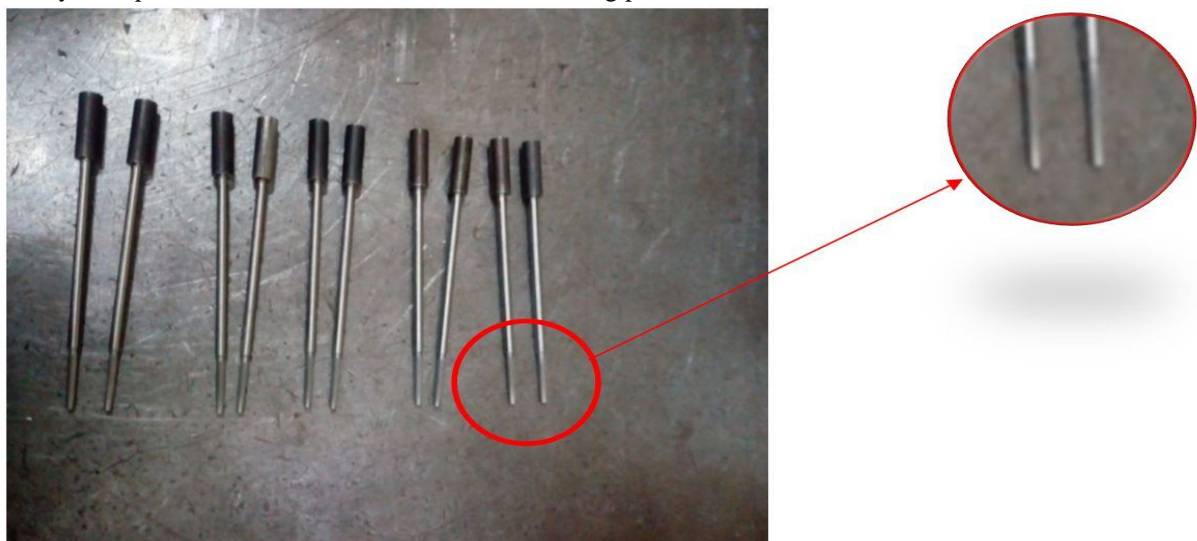
Fig 1: Core pins failure
