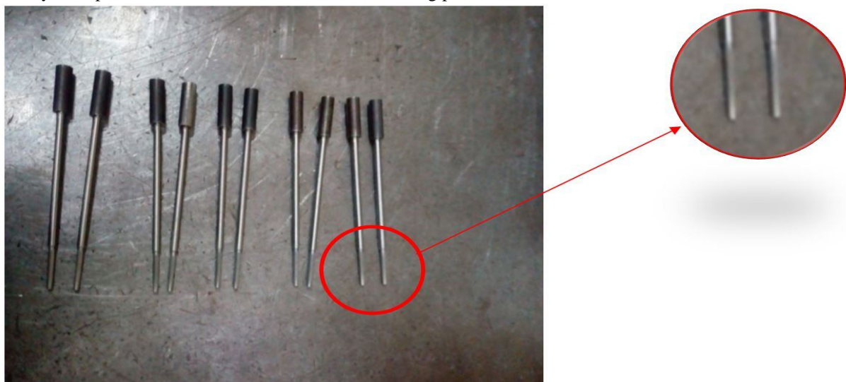
Fig 1: Core pins failure
