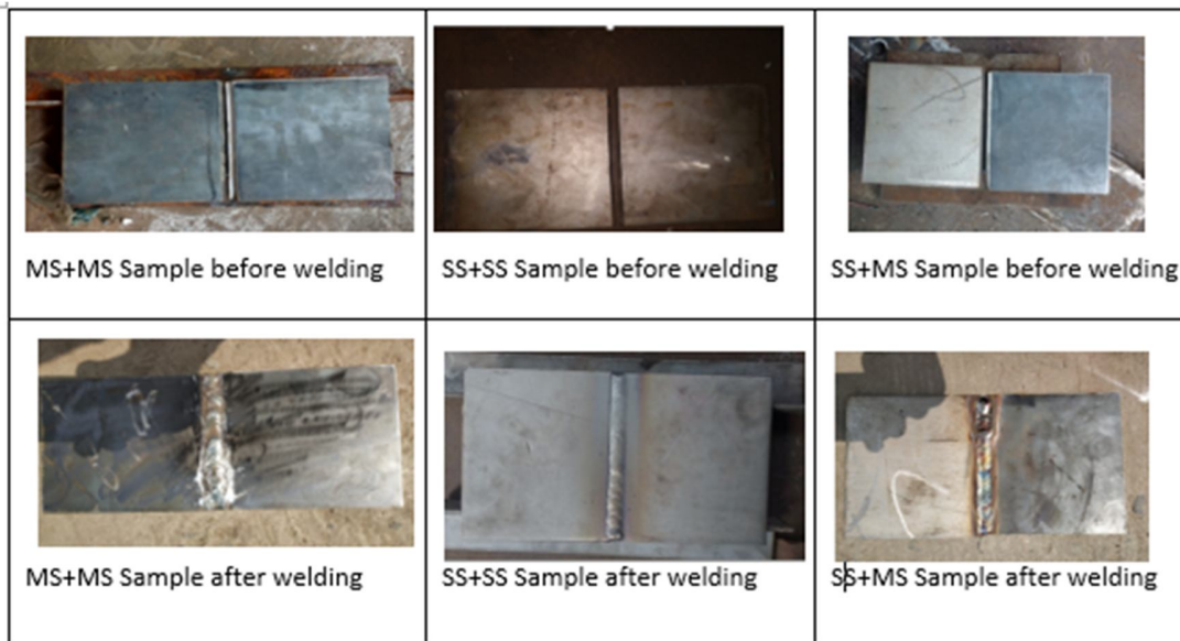
Fig: performance of welding
