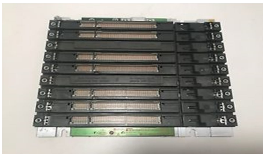
Fig.3. Simatic S7 400 universal rack with 9 slots
