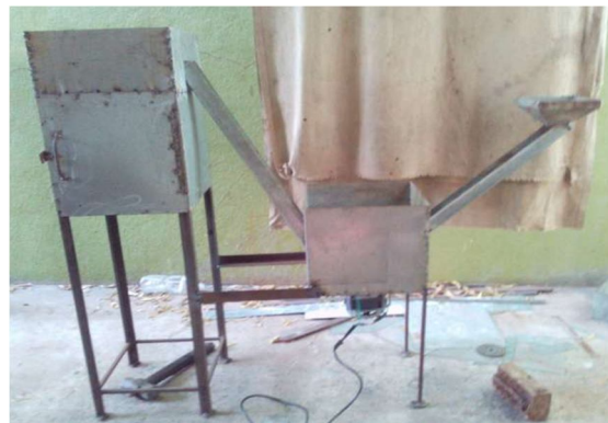
Fig 2 Waste plastic road making machine
