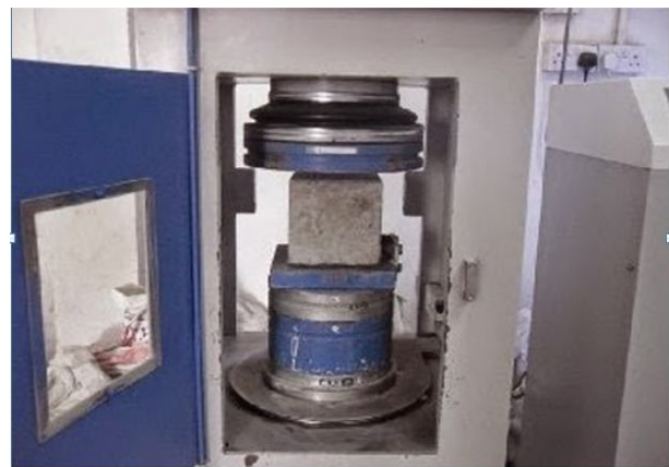
Figure 6: Compressive Strength Test
