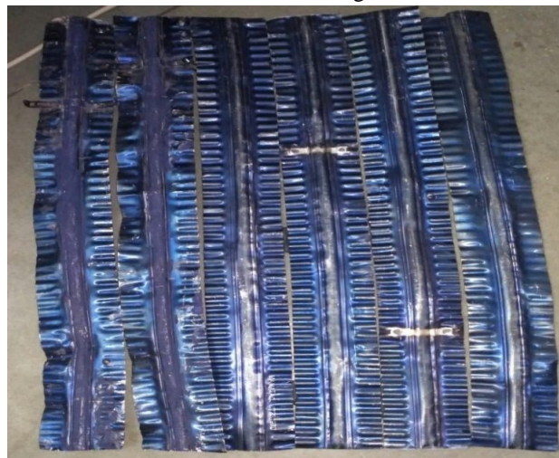
Fig 5. AIN with Blue Anti Reflective Coating on the Plate
