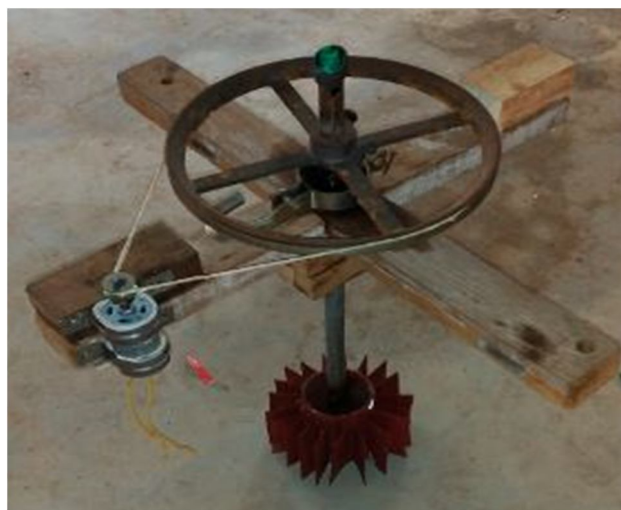
Figure: Blade and dynamo unit
