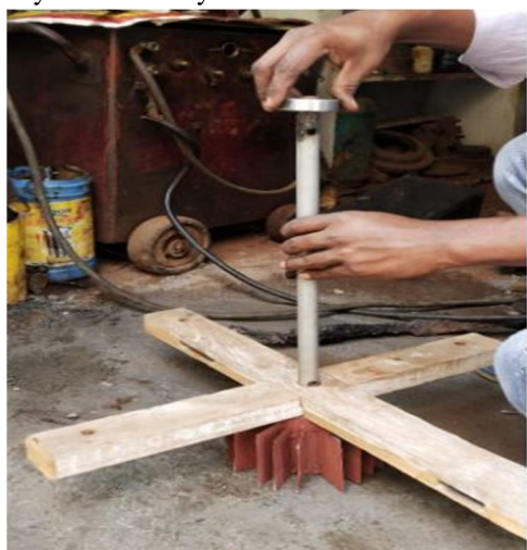
Figure: Fixing the wooden blocks and bearing to the shaft.
