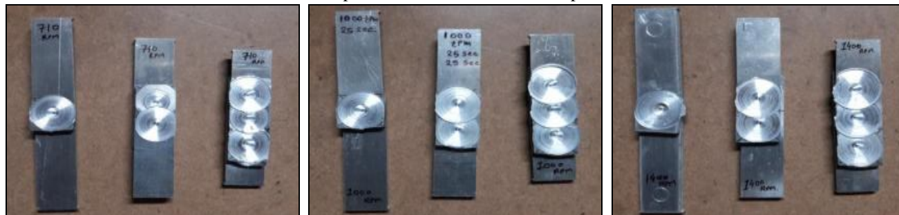
Fig.5 FSSW plates at 710RPM, 1000RPM and 1400RPM
