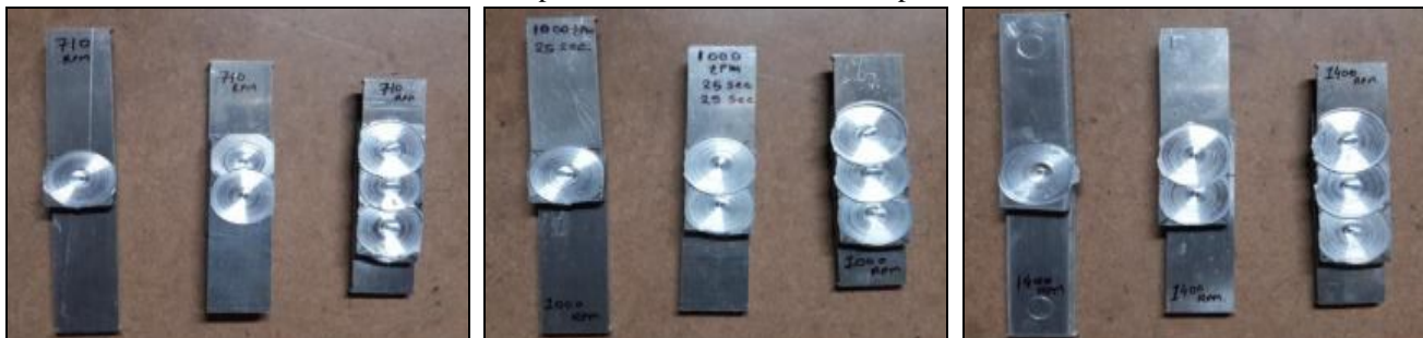
Fig.5 FSSW plates at 710RPM, 1000RPM and 1400RPM
