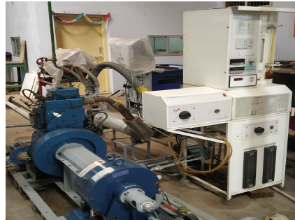
Fig. 6 Computerized variable compression ratio test rig.
