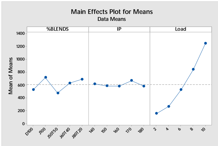
Figure 8 Main Effects Plot for Means of NO x Emission
