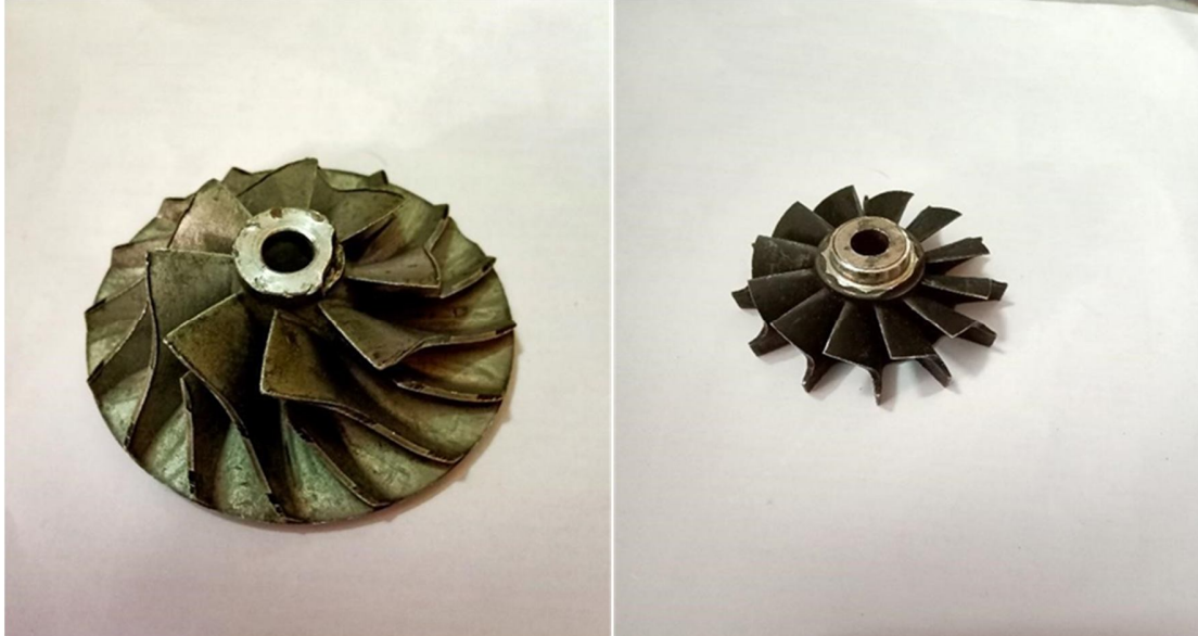
Fig. 8 Compressor And Turbine parts from the turbocharger
