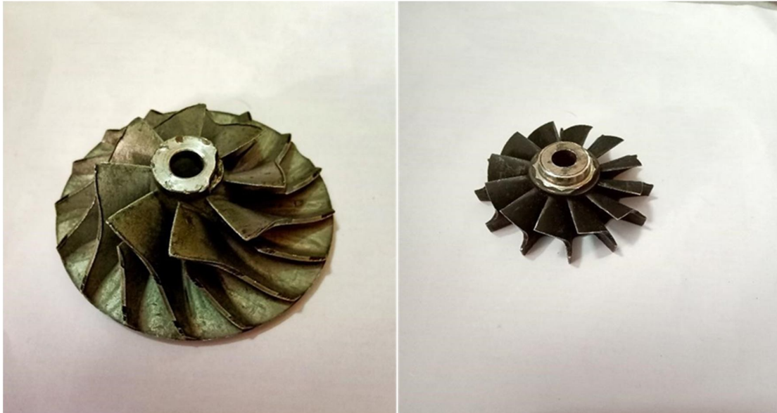
Fig. 8 Compressor And Turbine parts from the turbocharger
