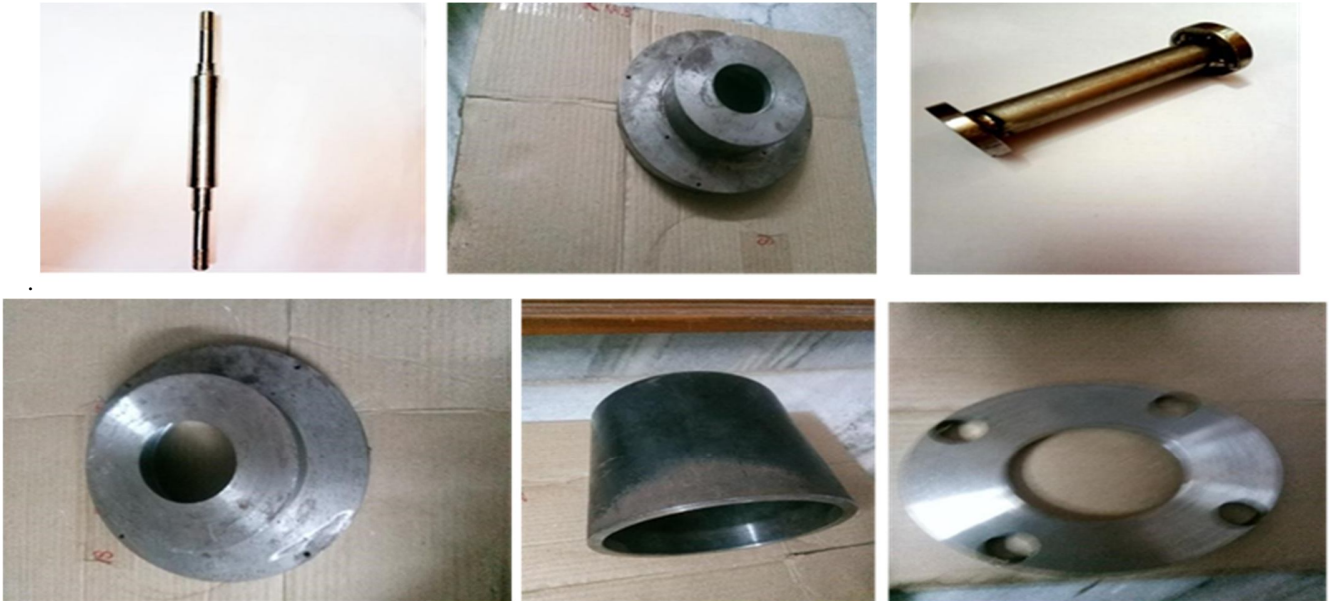
Fig. 11 The components which are produced on lathe
