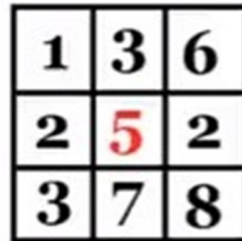
Figure 3 In each 3x3 block compare central pixel with 8 neighbours
