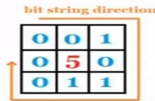
Figure 4 Selection of centre pixel and replacing binary values
