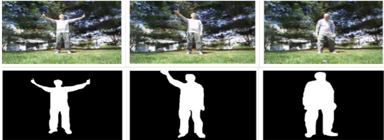
Figure 10 Comparison results on waving tree sequence, top row is the original frame sequence of 21 st , 25 th and 45 th frame. The first row indicates original frames and the second row indicates ground truth frames using MSTLBP
