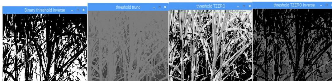
e) Binary threshold inverse f) Threshold trunc g) Threshold zero h) Threshold zero inverse
