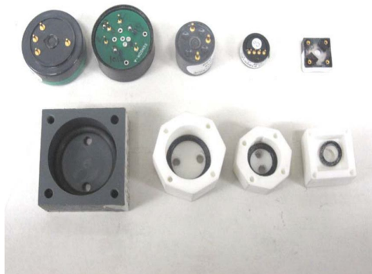
Figure 4.1. CO Electrochemical sensors and their isolation
