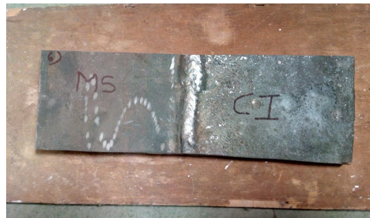
Photographs MS and CI plate butt joint
