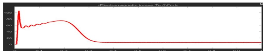
Fig.9: Response of torque of induction motor using seven level inverter
