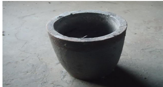
Fig.4.3: Graphite crucible used to keep molten metal in Muffle furnace
