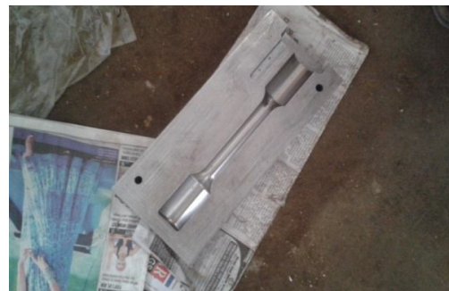
Fig.4.5: Die made up of Mild Steel
