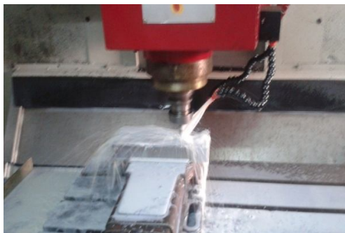
Fig.4.4: CNC used for preparing die
