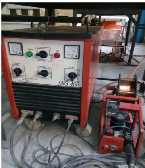
Figure 1: MIG Welding Setup
